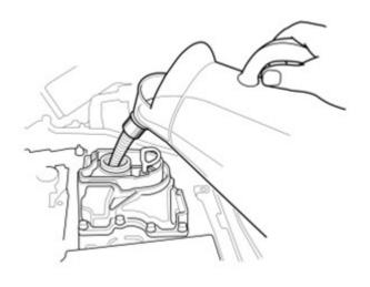
1. Refill the oil tank with the recommended engine oil to 6.5 L (6.9 US qt).
