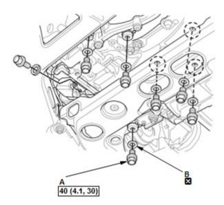
1. Remove the drain bolts (A), and drain the engine oil in sequence.
