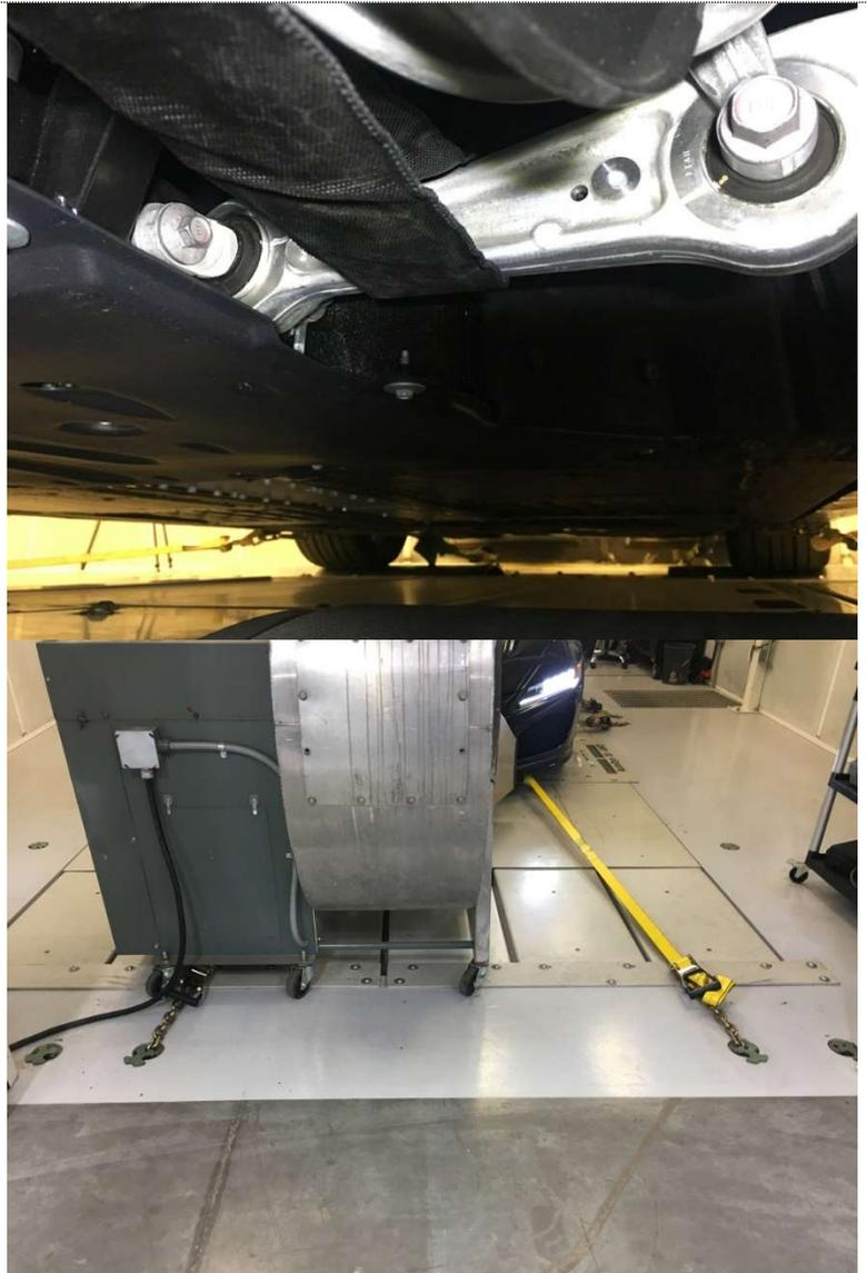
2. REAR: Place 1.5' long loop straps around rear lower control arm. IMPORTANT! Route strap under brake wire to prevent damage. Install 3' long ratchet strap chain in to inner floor mount pair.
