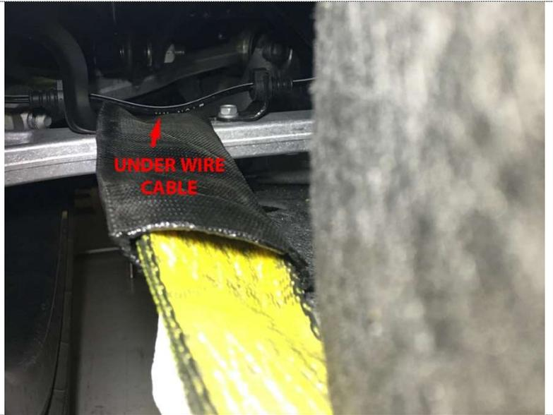
3. SIDE: Remove body plugs behind front wheels and in front of rear wheels & place in bag with brake duct hardware. Install mini-hooks in to body plug holes. Using 6' ratchet straps, secure as shown. IMPORTANT! Do not over torque – side straps are for stability and should be just-snug only.
